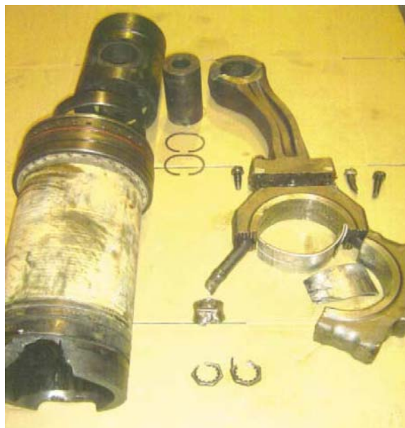
Fig. 3.15.1 Damaged piston liner and connecting rod
