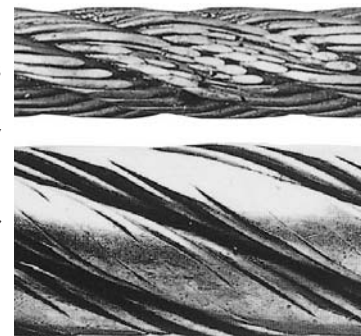
Example of abrasion failure
