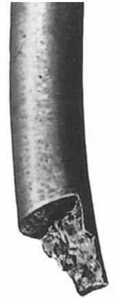
Example of fatigue failure
