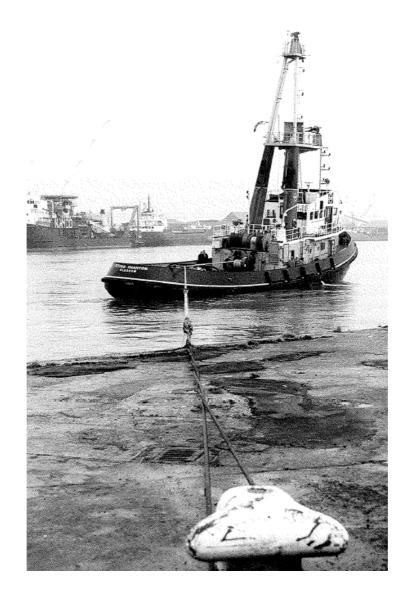
The achieved traction force is described as the "Continuous Bollard Pull" and has to differentiated from the so called "Static Bollard Pull".
