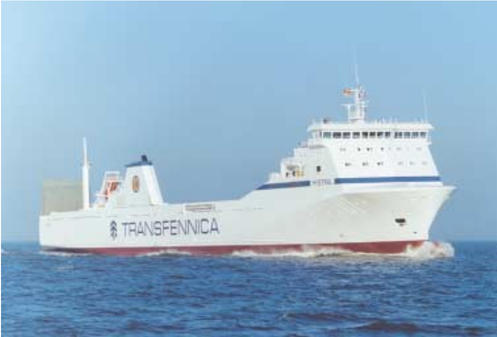
M/S Mistral delivered to Godby Shipping in January 1999 – one of the first of seven forest product carriers equipped with Direct Water Injection.
