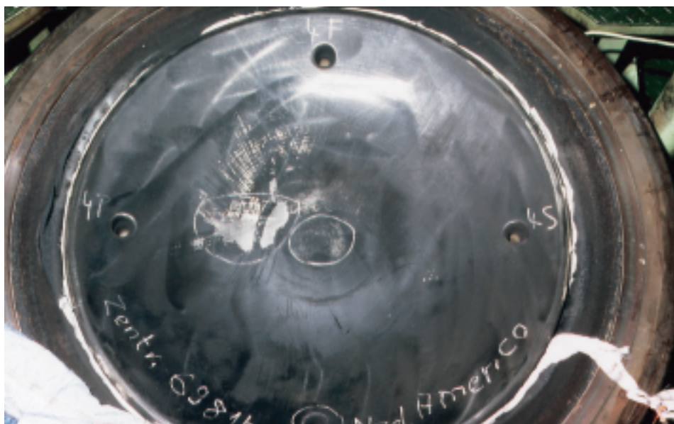
Fig. 37 Piston crown with a later test cladding from an 8RTA84C showing only minor attack after 6981 hours' operation [97#241]
