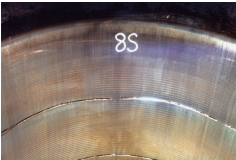
Fig. 51 Cylinder liner from the 12RTA84C engine of the Ever Ultra at 5019 hours' operation. The maximum diametrical liner ring wear is 0.04 mm/1000 hours [97#249]
