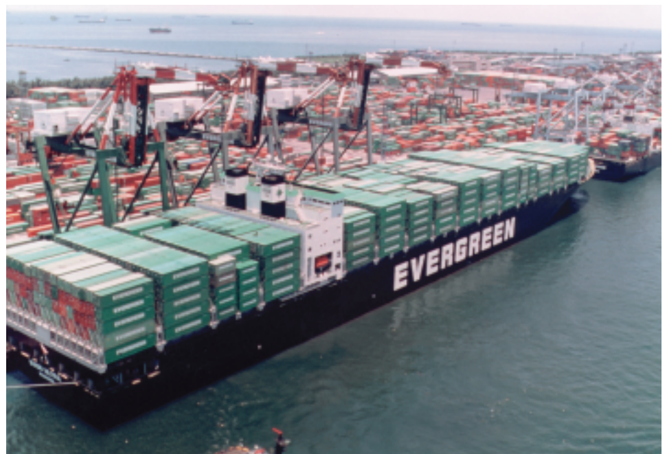
Fig. 9 The 5364 TEU Post-Panamax containership Ever Ultra powered by a 12RTA84C engine. Berthed ahead of her in Kaohsiung is the 2728 TEU Ever Grace of 1984 which has a Sulzer 6RLB90 main engine [7797-3027]
