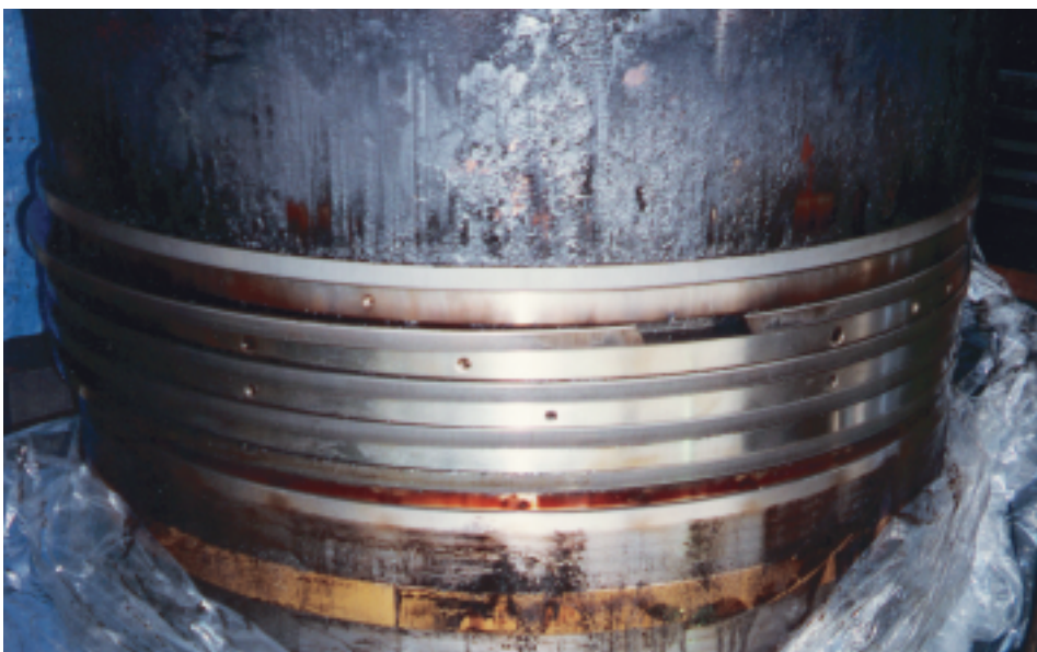
Fig. 56 Piston from the first 11RTA96C after 196 hours' running on the test bed [97#252]
