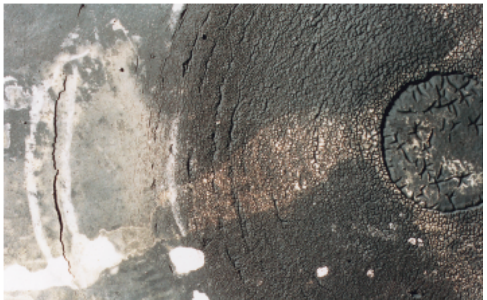
Fig. 36 Piston crown with test cladding from an 8RTA84C showing cracks in the cladding after 17 700 hours' operation [97#240]
