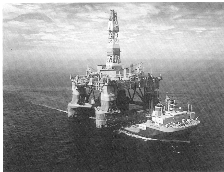
Fig. 1. Dry transport of the 19,000 T 'Ross' drilling rig
