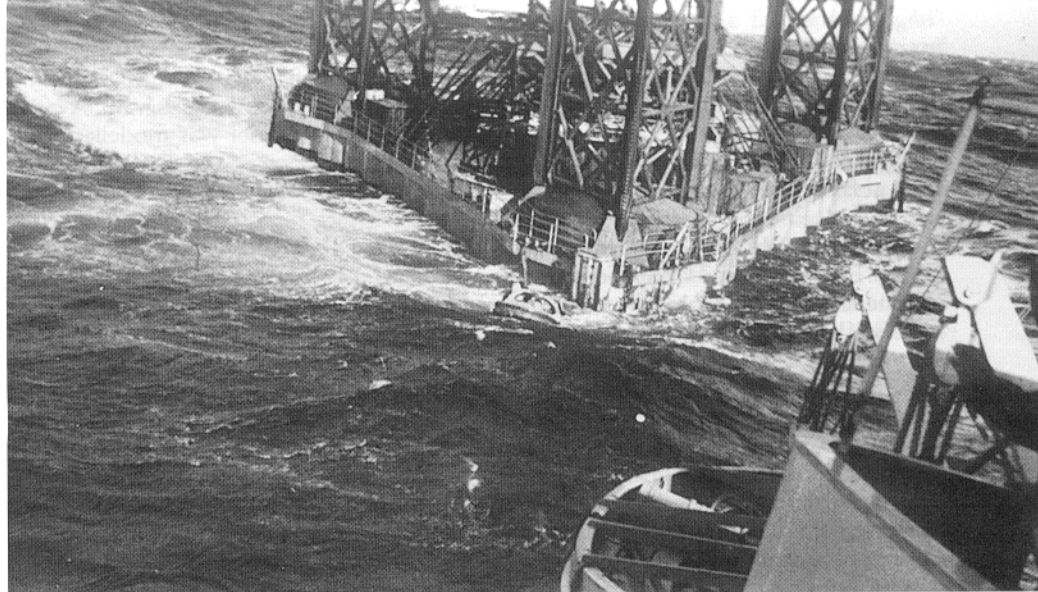
Fig. 2. 'Wet' tow of a jack-up drilling rig.
