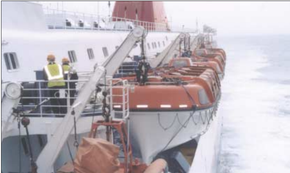
Typical lifeboat / davit installation
